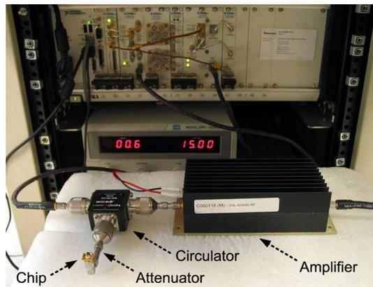
Fig. 6. Photograph of the testing setup with RFID chip connected.
