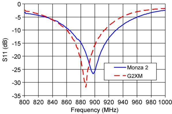
Fig. 10. Return loss of Monza 2 and G2XM RFID chip assemblies matched to 50 Ω.
