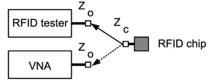
Fig. 2. Block diagram of the measurement setup.
