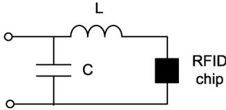
Fig. 9. Passive lossless LC-network used for matching chips to 50 Ω.
