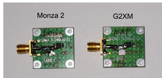
Fig. 8. Impinj Monza 2 and NXP G2XM RFID chip assemblies matched to 50 Ω.
