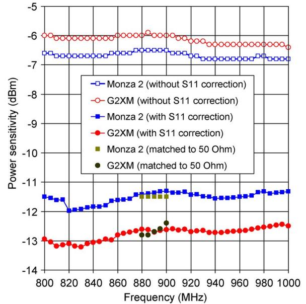
Fig. 7. Measured power sensitivity of RFID chips.
