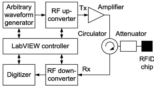
Fig. 5. Block diagram of RFID tester used in measurements.
