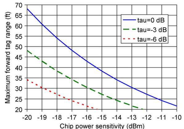
Fig. 1. Relationship between maximum RFID tag range (ft) and chip power sensitivity (dBm) for different values of power transmission coefficient. Other parameters: free space, 4-W EIRP, 915 MHz, 2-dBi tag antenna, perfect polarization match.
