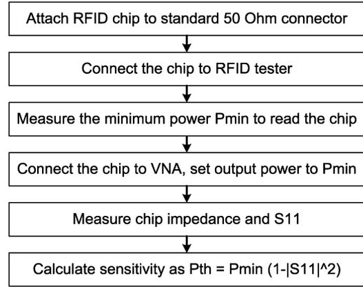
Fig. 3. Flow diagram of impedance and sensitivity measurements.
