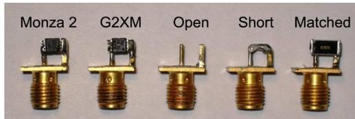
Fig. 4. Impinj and NXP RFID chips on 50-Ω SMA connectors.
