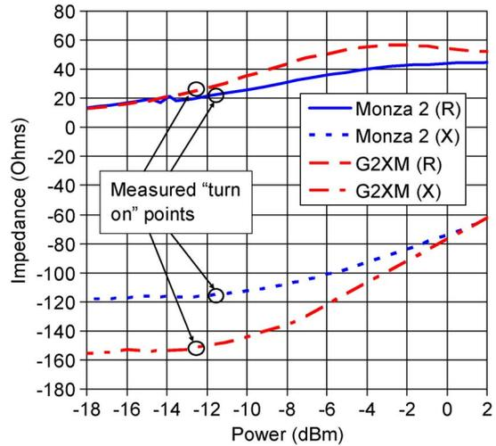
Fig. 12. Measured chip impedance versus absorbed power at 900 MHz.
