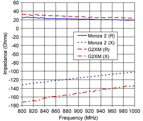
Fig. 11. Measured chip impedance versus frequency at the threshold power.
