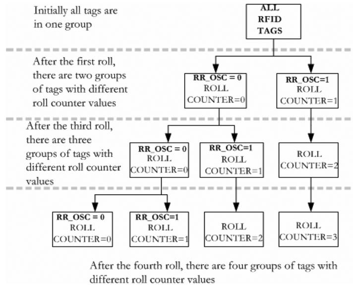
Fig. 14. Illustration of the binary sort algorithm.
