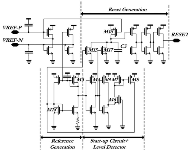
Fig. 7. Voltage reference, start-up circuit, and reset generation.
