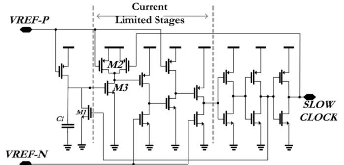
Fig. 2. Low-power oscillator that clocks the chip when it is in the “low-power” mode.
