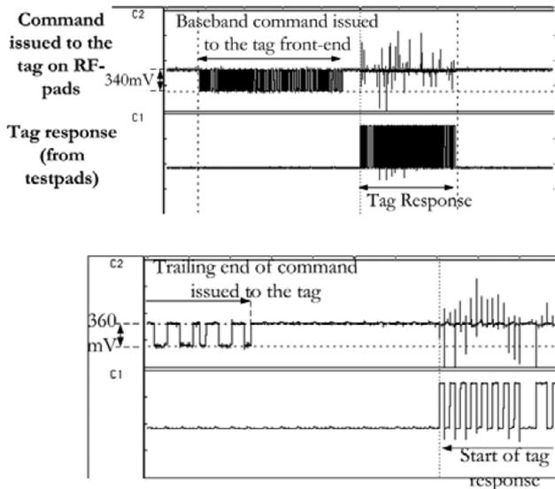
Fig. 19. Oscilloscope plots of baseband commands issued to the chip. Top shows a regular ISO-180006B command issued to the tag (after it is in the “full-power” mode) and the response of the chip (which is brought out on a testpad) is shown. Lower figure is a close up of the top figure showing portions of the command issued as well as the response from the chip.
