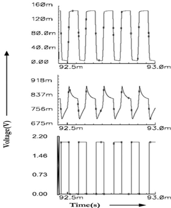
Fig. 6. Simulation results of the baseband amplifier. From top to bottom (a) Input square wave going into the baseband amplifier at node. (b) The differentiated signal at capacitor  $C1$ . (c) Output of the baseband amplifier.
