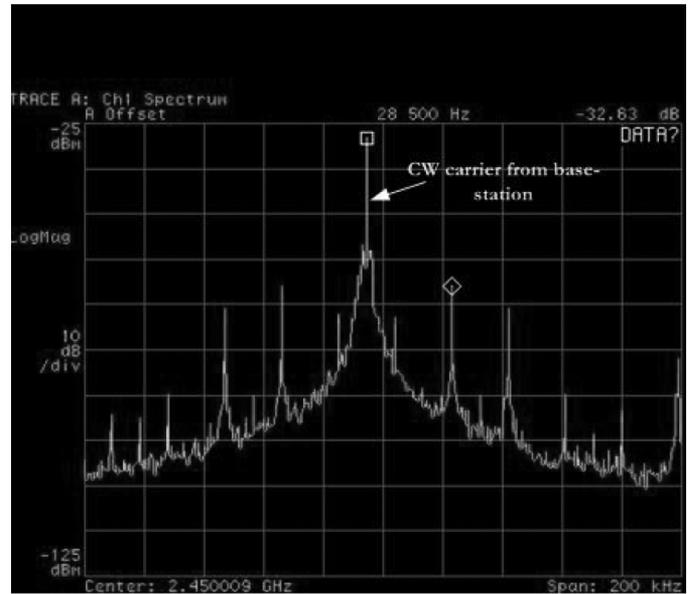
Fig. 21. Frequency spectrum of the tag response measured with an HP-89441A, using a RBW = 1 kHz. The tag is located 11 in away from the base-station with an inline attenuation in the forward path of 11 dB.
