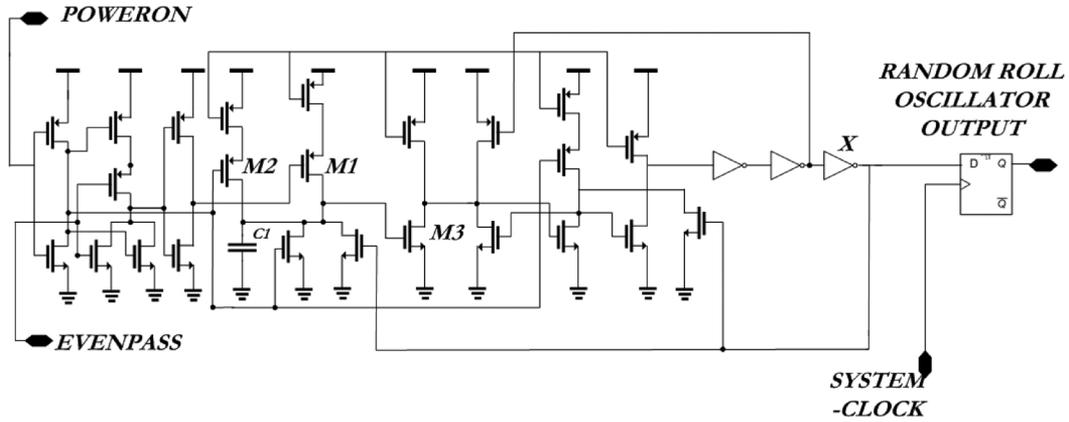
Fig. 13. Circuit schematic for the random roll oscillator which is used for generating random bits for the binary sort algorithm.
