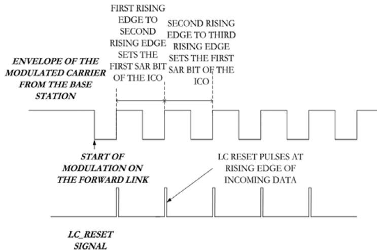
Fig. 12. Calibration of the clock recovery block to the incoming command from the base station. The lower figure shows the generation of the *LC\_RESET* signal that is used to reset the phase of the oscillator as well as to reset the digital section to the next round of calibration.
