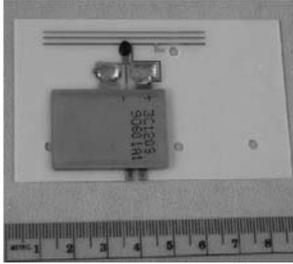
Fig. 18. Photograph of the assembled tag (chip wire-bonded and globbed to FR404 substrate) with a thin battery attached.
