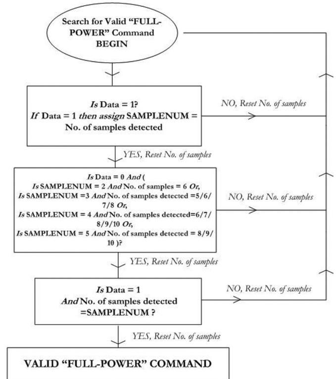
Fig. 15. Algorithm implemented by the signal processing state machine. SAMPLENUM is the number of samples detected during the first bit period, data is sampled incoming data and the number of samples is reset at every block transition.
