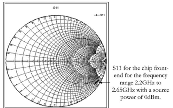
Fig. 22. S11 plot for the chip front-end, measured with an HP8719C vector network analyzer.
