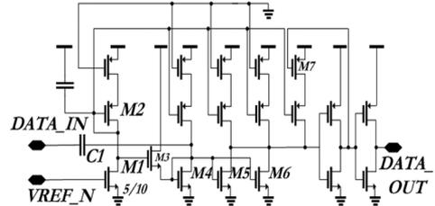
Fig. 5. Baseband amplifier circuit schematic.
