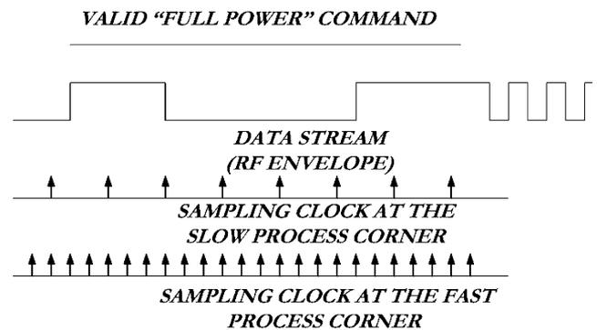
Fig. 16. Sampling of incoming command when the oscillator runs slow and when the oscillator runs fast.
