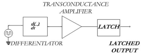
Fig. 4. Baseband amplifier architecture.
