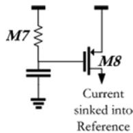
Fig. 8. Equivalent circuit for start-up circuit at power-up.
