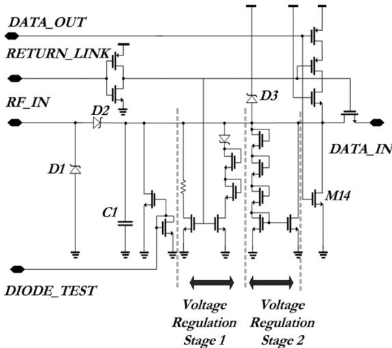
Fig. 3. RF front-end on the chip with the voltage regulators and the modulator for back-scattering.
