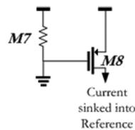
Fig. 9. Equivalent circuit for start-up circuit when the supply voltage is less than 1.3 V.
