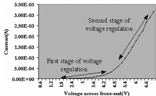
Fig. 23. Experimentally measured  $I-V$  characteristics of the front-end. The  $I-V$  curve shows the regions where the two stages of voltage operate.
