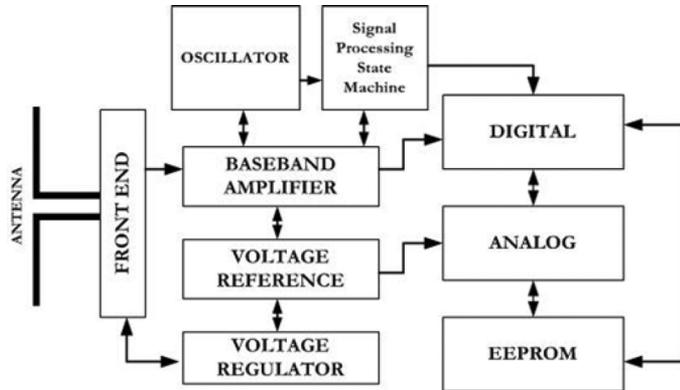
Fig. 1. Block diagram of the whole chip.
