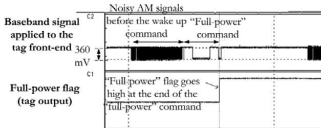
Fig. 20. Oscilloscope measurements of a series of bit patterns issued to the chip. Note that the chip does not falsely decode any of the bit streams as a “full-power command” and correctly decodes the “full-power” command.
