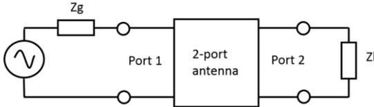
Figure 14. Equivalent circuit of the self-reconfigurable antenna.
