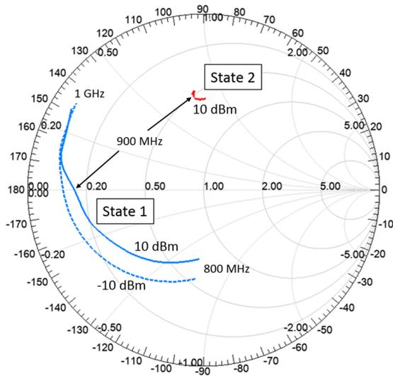
Figure 5. Two impedance states of the switching circuit.
