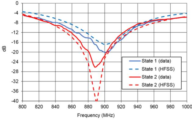
Figure 13. Measured and simulated S11 of the antenna in two states specified in Table I.
