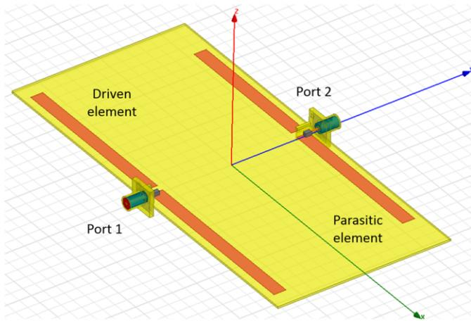
Figure 8. Antenna model in HFSS.
