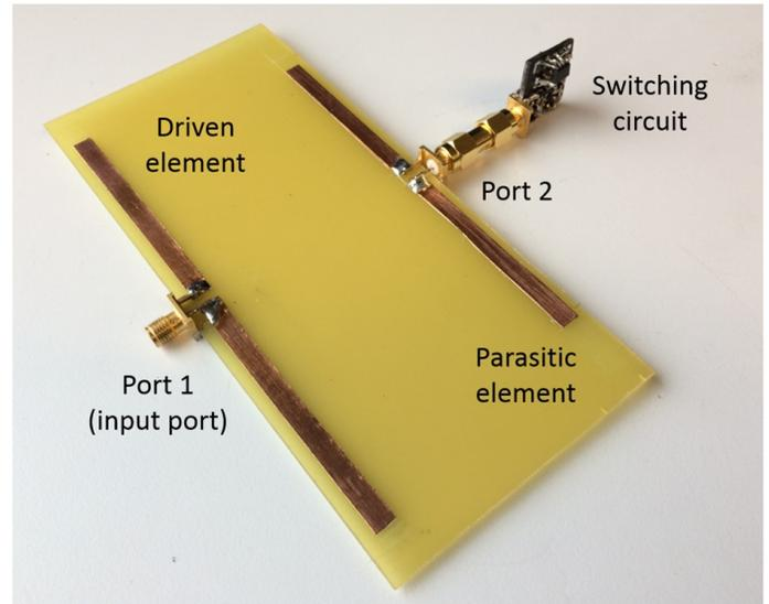
Figure 11. Prototype antenna.
