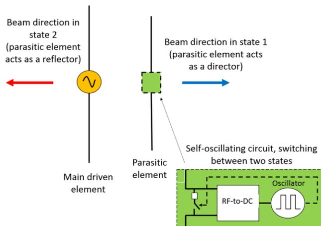
Figure 1. Self-reconfigurable 2-element Yagi antenna with switching circuit on parasitic element.
