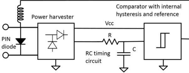
Figure 2. Block diagram of the switching circuit.
