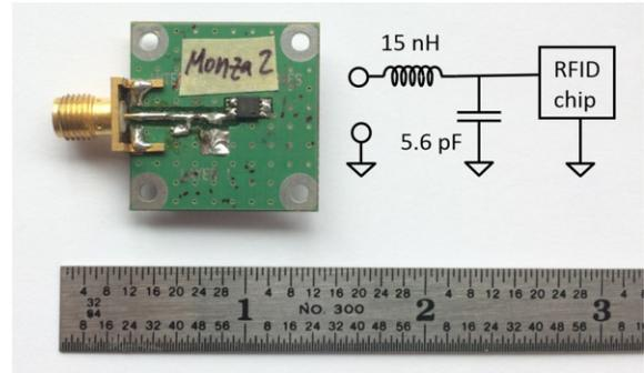
Figure 17. Conducted tag used for pattern measurements.
