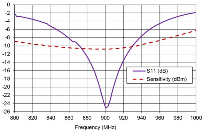
Figure 18. Threshold power sensitivity (dBm) and return loss (dB) of the conducted tag.
