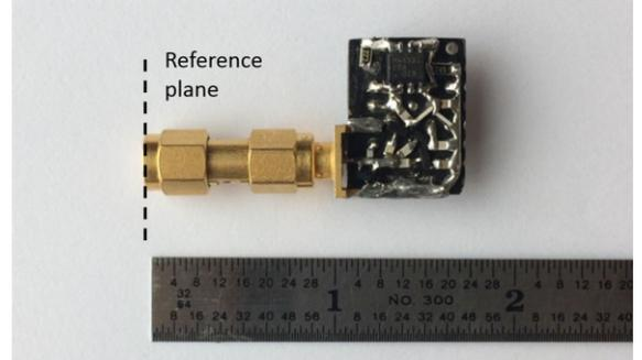
Figure 4. Switching circuit prototype.
