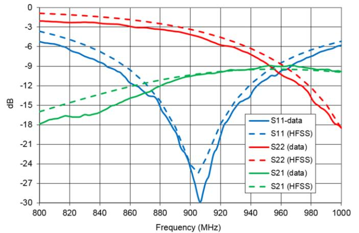
Figure 12. Measured and simulated S-parameters of the antenna.
