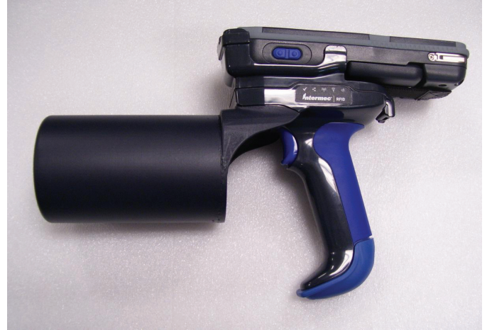
Fig. 8. Prototype of antenna described in Table II, shown attached to the handheld UHF RFID reader with mobile computer.
