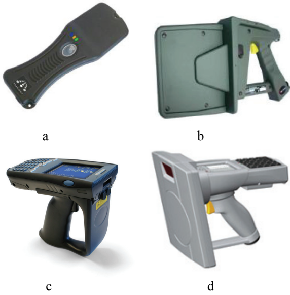
Fig. 2. Examples of antennas used in commercial handheld UHF RFID readers: a – Tracient [6], b – IPICO [7], c – Unitech [8], d – Skeye [9].
