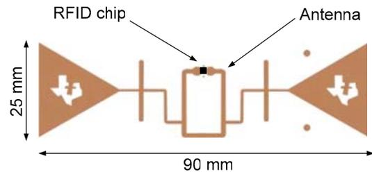
Fig. 8. UHF RFID tag used in measurements.
