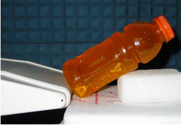
Fig. 13. Gen2 UHF RFID tag inside the bottle of sports drink being read using standard far-field UHF RFID antenna.
