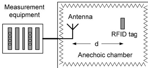
Fig. 4. Measurement setup.
