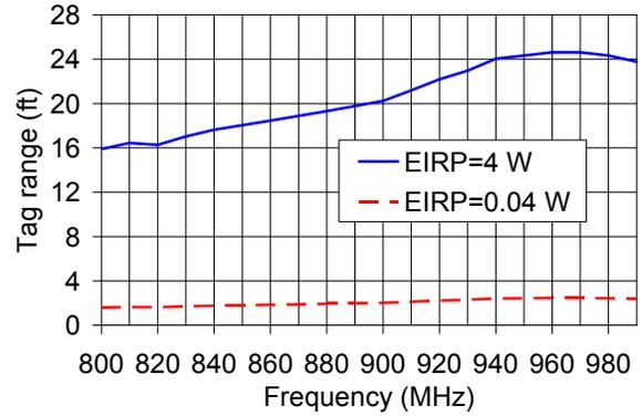
Fig. 11. Tag range vs. frequency for different EIRP values.
