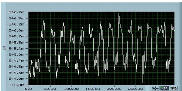
Fig. 15. Portion of the received tag response at 890 MHz with the reader output power of 24 dBm in the scenario shown in Fig. 13.
