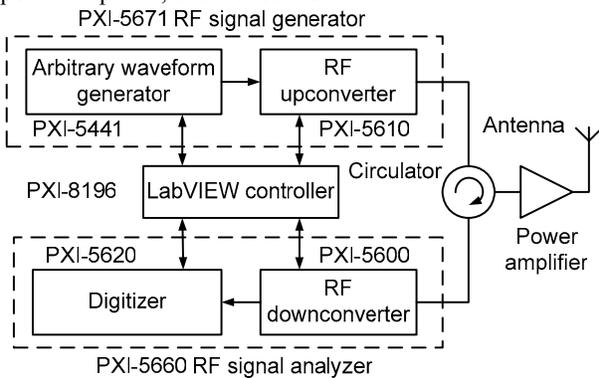
Fig. 5. Measurement equipment block diagram.
