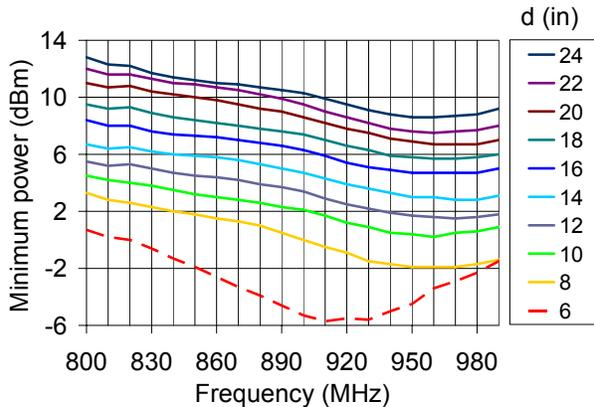
Fig. 10. Minimum power vs. frequency for various distances between the tag and the reader antenna.
