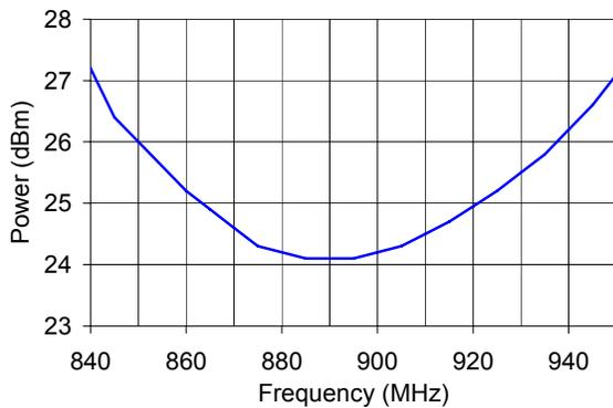
Fig. 14. Minimum reader output power vs. frequency necessary to read the tag in the scenario shown in Fig. 12.
