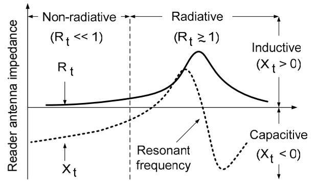
Fig. 3. Different regions of reader antenna impedance (shown for a typical dipole antenna).
