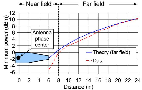
Fig. 12. Minimum power vs. distance at 900 MHz.
