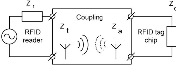
Fig. 2. Antenna coupling in general RFID system.
