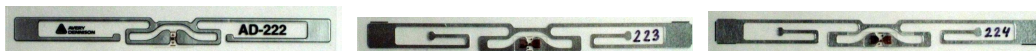
Figure 2. Tags used in measurements, left to right: AD-222 (Impinj Monza 2 IC), AD-223 (Impinj Monza 3 IC), and AD-224 (NXP G2XM IC).
