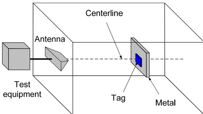
Fig. 10. Experimental setup for measuring the read range of the tag on metal (normal and lateral) for 4 W EIRP.
