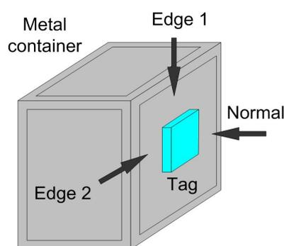
Fig. 2. Required normal and edge readings of the container tag.
