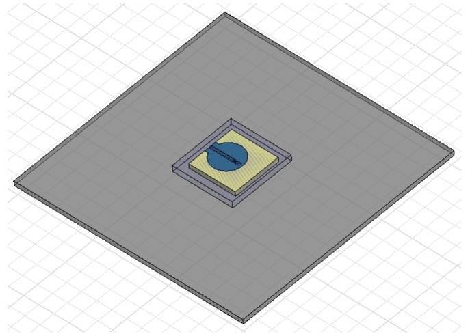
Fig. 5. Geometry used in HFSS simulations: encapsulated tag placed on 30 cm x 30 cm sheet of metal.
