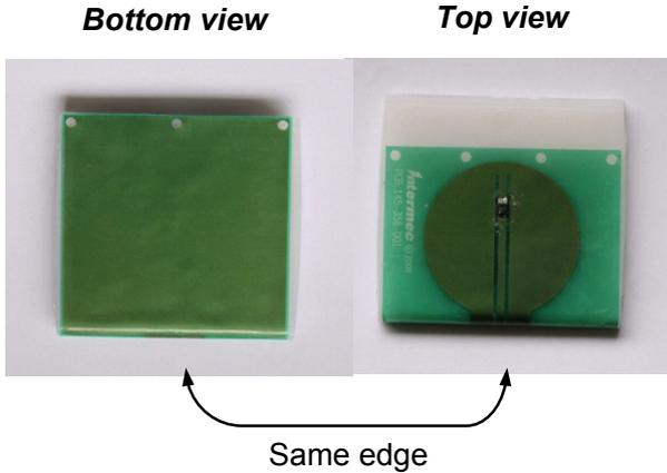
Fig. 8. Photograph of the tag prototype made with the inlay wrapped around the dielectric.
