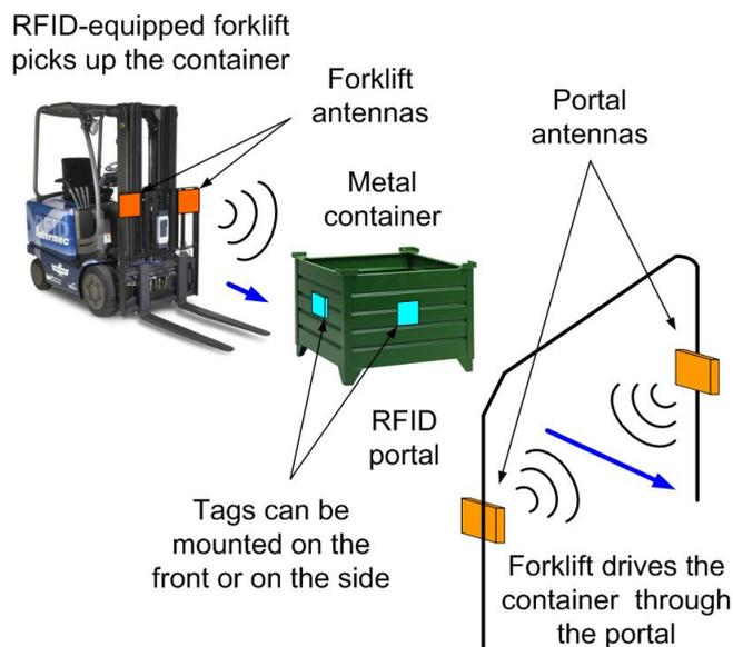
Fig. 1. Application scenario for metal container tag.
