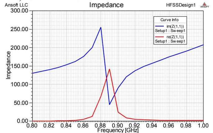
Fig. 7. Simulated complex antenna impedance vs. frequency.
