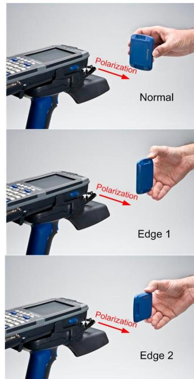
Fig. 12. Illustration of the tag reading directions using handheld RFID reader with linearly polarized antenna.
