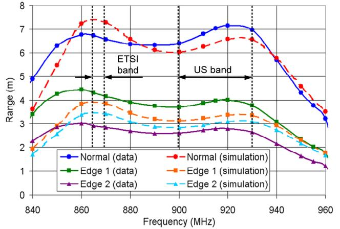
Fig. 11. Experimental read range of the tag on metal (normal and lateral) for 4 W EIRP (two RFID bands, ETSI and US are shown).
