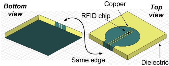
Fig. 3. Tag structure (general view).
