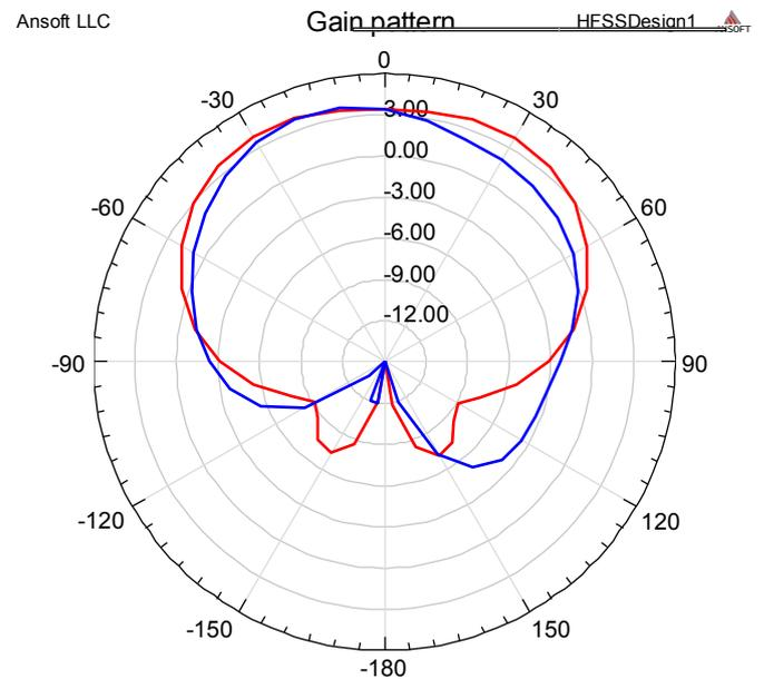
Fig. 6. Simulated gain pattern (E-plane, red color, and H-plane, blue color) at 900 MHz. The scale is in dB.
