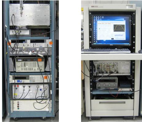
**Figure 8 – Intermec RFID test systems: left - custom system (1997), right - NI PXI system (2007).**
