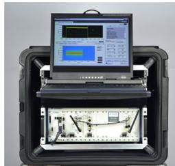
**Figure 9 – Nexjen NI PXI RFID test system (image from [32]).**
