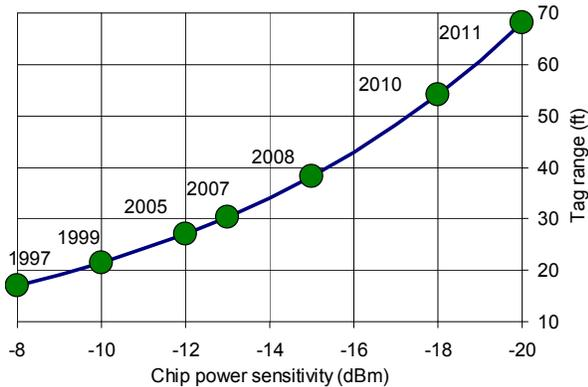
Figure 2 – Tag read range vs. chip sensitivity (4 W EIRP, free space, 915 MHz, 2 dBi matched tag).
