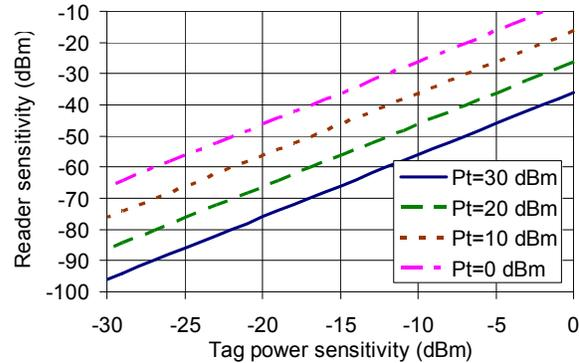
Figure 4 – Reader sensitivity needed to read tags of different sensitivity at their maximum possible range. The tag backscatter gain is assumed to be -10 dB.
