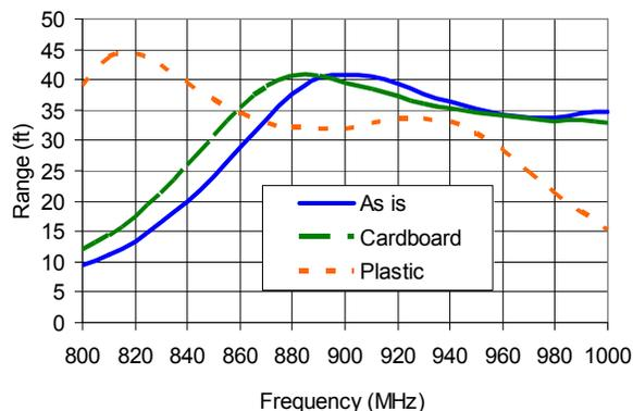
Figure 15 - Read range of AD-223 tag on different materials (4 W EIRP, free space).
