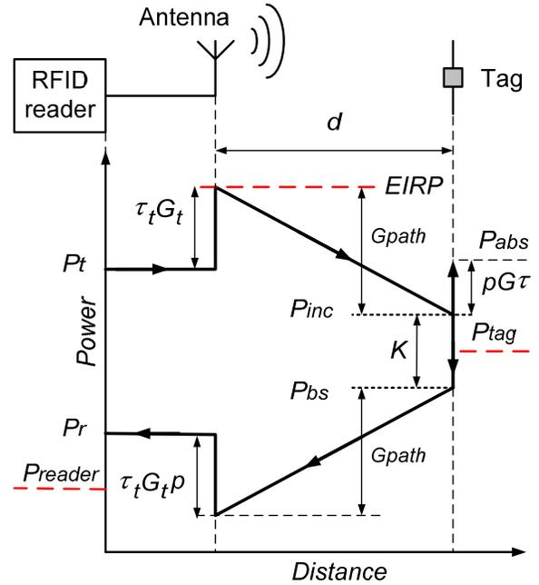
**Figure 1 – RFID system link budget diagram.**
