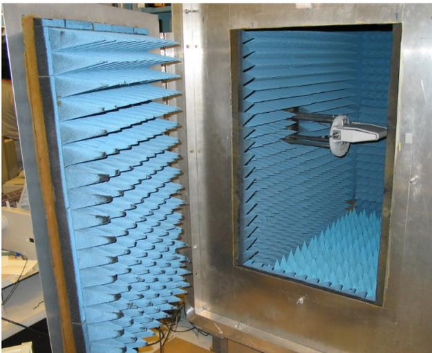
Figure 5 – Anechoic chamber used for tag measurements at Intermec.
