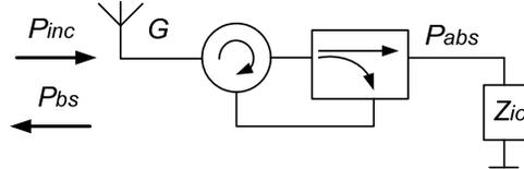
Figure 3 – Simple RF model of RFID tag.
