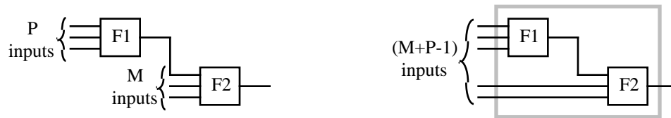
Figure 71. Example for the discussion of the size of logic functions. The P -input and M -input functions cascaded together (left) are fit into a (M+P-1) input LUT (right).
