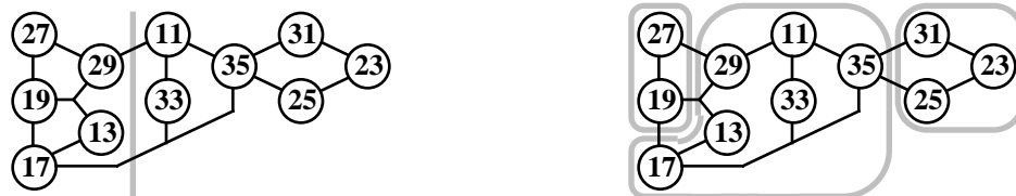
Figure 72. Example of the impact of technology-mapping on partitioning quality. The circuit s27 is shown (clock, reset lines, and I/O pins are omitted). At left is a balanced partition of the unmapped logic, which has a cutsize of 2. Gray loops at right indicate logic grouped together during technology-mapping. The only balanced partitioning has the largest group in one partition, the other two in the other partition, yielding a cutsize of 5.
