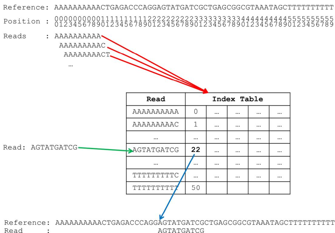
**Figure 7: Simple indexing solution shows the creation of the index table (red) by walking along the reference and recording the reads that appear at every location in the index table. Short reads are used as an address into the index table (green), and the final alignment for the read is read from the index table (blue).**
