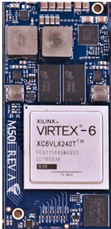
Figure 13: M501 board from Pico Computing, with the Virtex-6 FPGA visible from the top view. [20]
