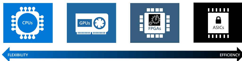
Figure 2: Silicon alternatives from most flexible (left) to most efficient (right), including CPUs, GPUs, FPGAs, and ASICs. TPUs (not pictured) are a relatively new development, which have flexibility similar to GPUs, but may have higher efficiency for ML inference. Figure adapted from Ref. [57].
