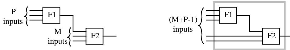
Figure 2. Example for the discussion of the size of logic functions. The P -input and M -input functions cascaded together (left) are combined into a (M+P-1) input LUT (right).
