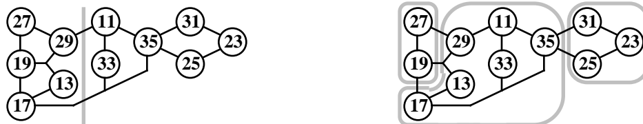
Figure 3. Example of the impact of technology-mapping on partitioning quality. The circuit s27 is shown (clock, reset lines, and I/O pins are omitted). At left is a balanced partition of the unmapped logic, which has a cutsizes of 2. Gray loops at right indicate logic grouped together during technology-mapping. The only balanced partitioning has the largest group in one partition, the other two in the other partition, yielding a cutsizes of 5.
