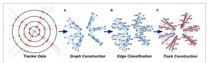
FIGURE 2 | High-level overview of the stages in a GNN-based tracking pipeline. Only a subset of the typical edge weights are shown for illustration purposes. (A) Graph construction, (B) edge classification, and (C) track construction.
