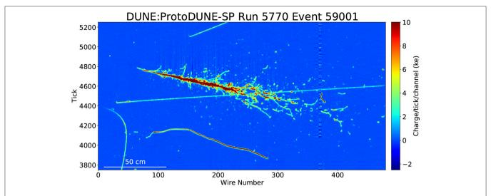
FIGURE 4 | A 6 GeV/c electron event in the ProtoDUNE detector. The x-axis shows the wire number. The y-axis shows the time tick in the unit of 0.5μs. The color scale represents the charge deposition.
