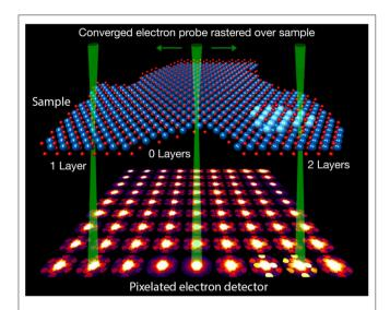
**FIGURE 5** | Experimental 4D-STEM measurement of a dichalcogenide 2D material. Atomic map is inferred from the data, each diffraction pattern represents an average of  $7 \times 7$  experimental images, green STEM probes are labeled for regions of the sample with one layer, vacuum, and two layers (Ophus, 2019).
