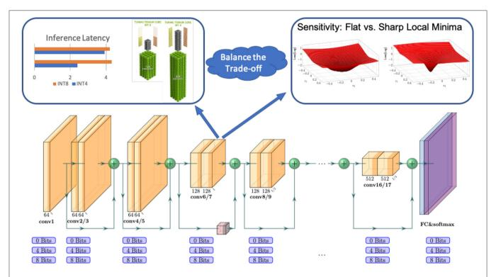
**FIGURE 6** | The illustration of hardware-aware quantization and pruning. A given NN model can be compressed by using low precision quantization instead of single precision. The extreme case is to use 0-bit quantization which is equivalent to removing/pruning the corresponding neurons. The goal of compression is to find the best bit-precision setting for quantization/pruning to reduce model footprint/latency on a target hardware with minimal generalization loss.
