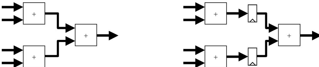
**Figure 3.1: Clock Frequency and Latency Effects of Pipelining**
