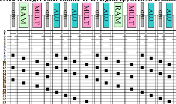
Figure 1: Block diagram of one full-custom RaPiD II cell. Up to thirty of these cells are placed along the horizontal axis. Data flows through the array along the horizontal axis in both left-to-right and right-to-left directions, with vertical routing providing connections between functional units. The black boxes in the interconnect represent bus connectors, which can be used to connect tracks into long lines or to separate them into short lines.
