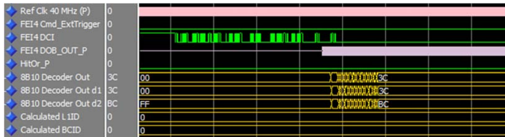
Figure 4.3: Prior to sending triggers or injecting hits into the FE-I4, the front-end model must be configured and put into run mode. The correct set up of the testbench is indicated by a continuous output stream on the serial DOB_OUT_P signal. After this signal is decoded by the BOC CDR and 8b/10b decoder, the signal would stabilize at the DC-balanced hexadecimal “3c.” Some junk data is generated by the FE-I4 right after its initialization which must be discarded prior to any data-taking tests.
