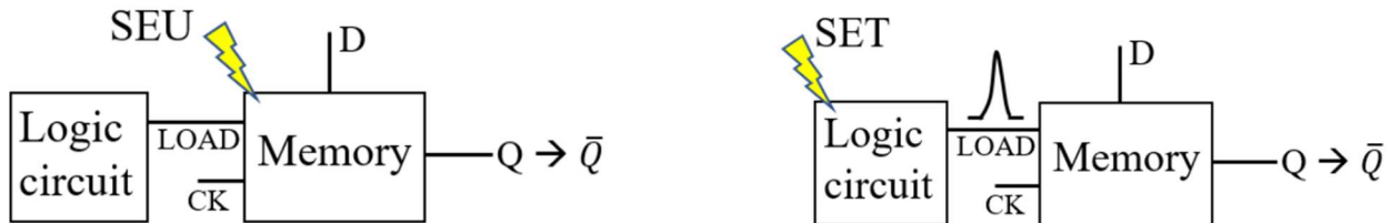
Figure 7: Schematic image of SEU (left) and SET (right) [18]
