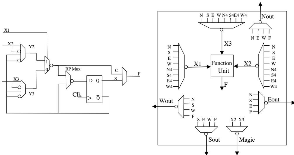
Figure 4. XC6200 Function Unit and Cell Routings.
