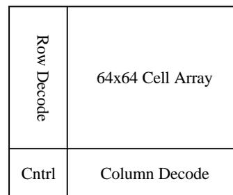
Figure 1. XC6216 simplified block diagram.
