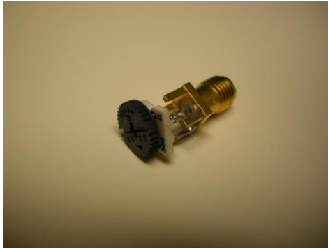
Figure 6. The variable 500 \Omega potentiometer load.
