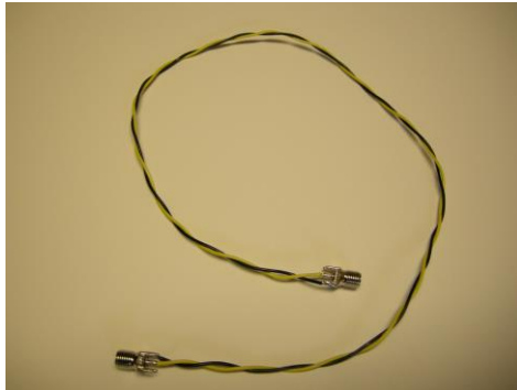
Figure 7. An 18 inch section of twisted pair line with female SMA connectors.
