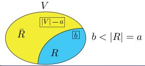
• Can use this to define a truncated matroid rank function. With  $r(A) = \min(|A \cap R|, b) + |A \cap \bar{R}|, b < a$ , define:
