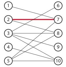
Any edge, not intersecting nodes adjacent to current matching is an augmenting path.
