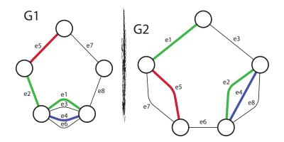
Removing blue and adding green leads to higher cardinality independent set in both matroids. This corresponds to doing  $I \leftarrow I \ominus S$  where  $S = (e_2, e_4, e_1)$  and  $I = \{e_4, e_5\}$ .
