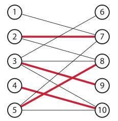
At this point, resulting alternating path is not augmenting, since it is not between two unmatched vertices (and no augmenting path is possible).
