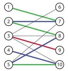
At this point, resulting alternating path is not augmenting, since it is not between two unmatched vertices (and no augmenting path is possible). At this point, matching is maximum cardinality.
