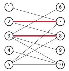
No possible further single edge addition at this point. We need a multi-edge augmenting path if it exists.
